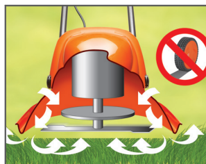
Air cushion Floats on a cushion of air.
